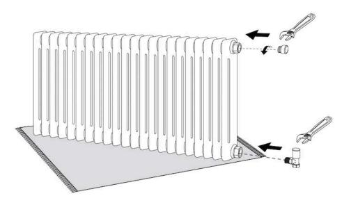
Apply PTFE tape to valves and screw into bottom of radiator tighten with a spanner.
