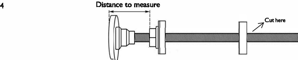
Measure the distance from the wall to where the back of the radiator is to sit, as shown above. The Clamping Plate can be used in either a vertical or horizontal position. Radiators with a smaller space between each section, the Clamping Plate should be positioned Vertically. Radiators with a larger space between each section, the Clamping Plate should be positioned horizontally. Install the red washer, then the Thistle head will screw through the un-threaded clamping plate.
